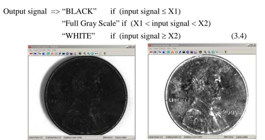
Figure 3.3 – Original and processed image with threshold and gray scale stretch.
