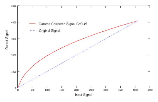
Figure 2.14 – Gamma corrected video signal.
