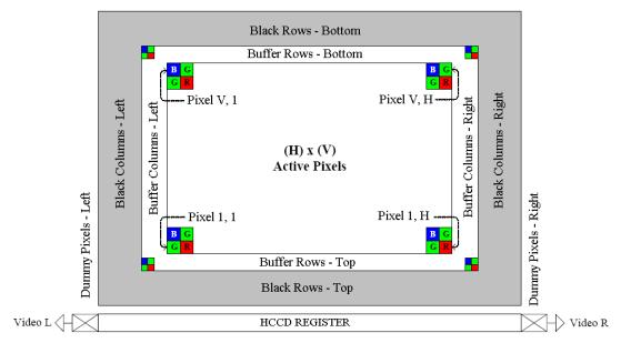
Figure 1.1– Interline CCD Pixel Structure.
