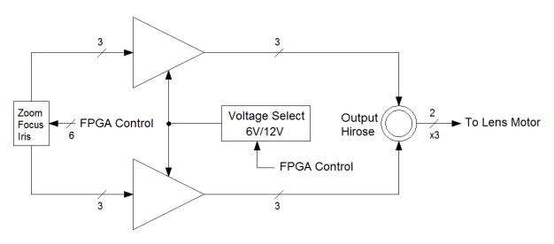
Figure 2.12 – Lens Control output electrical connection.
