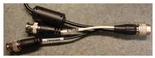
Trigger & Strobe pigtail with Male BNC connectors
