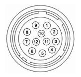
Figure 1.10 – HD-SDI Camera Serial/Lens Control Pin-Outs (Rear view)
