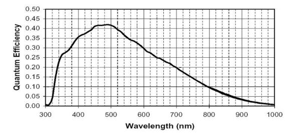
Figure 1.2 – KAI (TRUESENSE) CCD typical mono spectral response (Monochrome with the cover glass).
