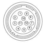
Figure 1.9 – HD-SDI Camera Power Connector Pin-Outs (Rear view).
