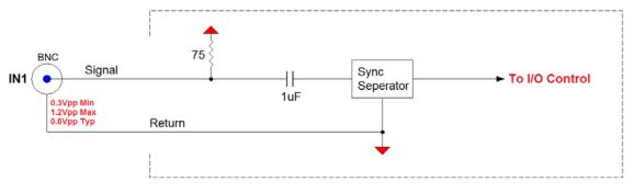
Figure 2.10 – IN1, Tri-Level Sync electrical input connection.
