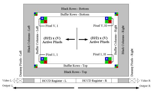
Figure 2.1– Dual output mode of operation.
