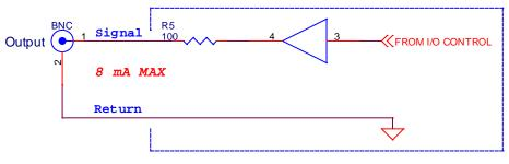
Figure 2.11–OUT1, OUT2 electrical connection.
