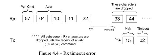
**Example**: Write to register address 0x0410, data value = 0x11223344:  $\Rightarrow$  Camera Write Command : <0x57> <04> <10> <11> <22> <33> <44>
