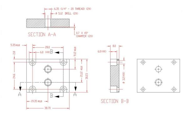
Figure 1.14 – HD-SDI mounting plate using ¼ in 20 thread.
