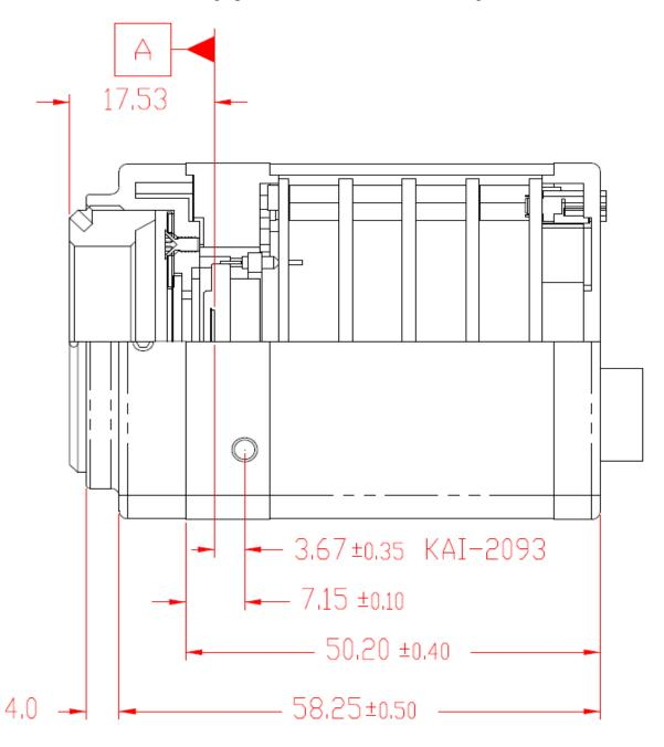
Figure 1.15 – Optical plane position for the SDI-B1920M, B1920C.
