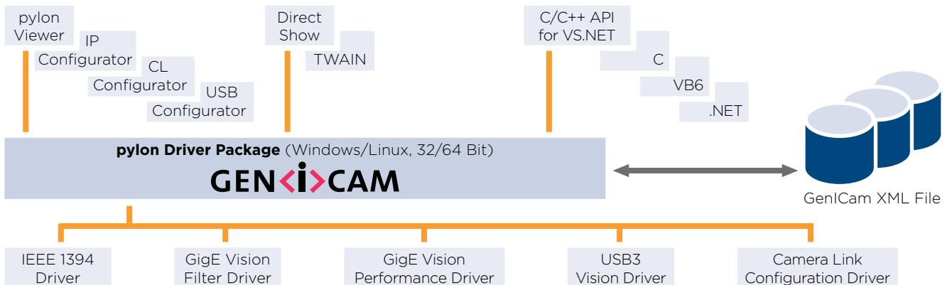
The internal architecture of the pylon driver package is based on GenICam Technology, which offers you easy access to the newest camera models and the latest features. Changes to an existing camera device in your application essentially become a plug-and-play process.
