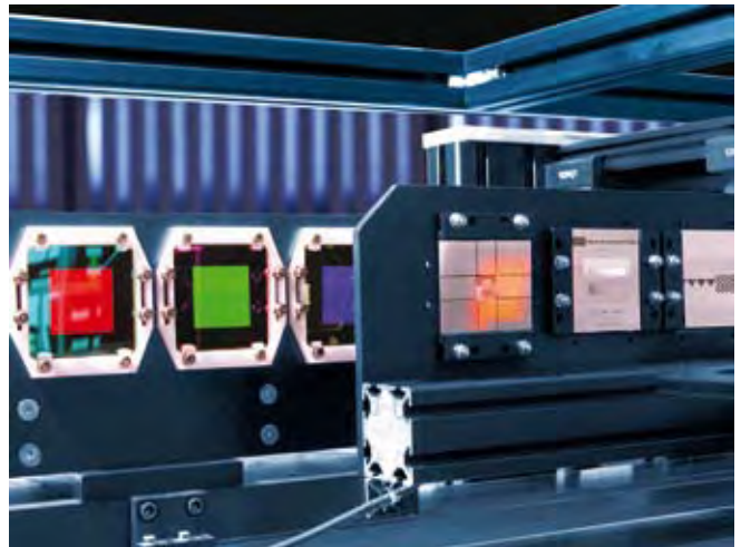
The A630f and A640f are measured by the CTT+ according to the EMVA 1288 standard
