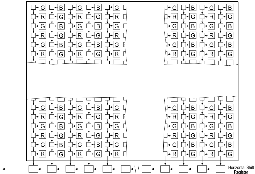
Figure 3-10: Bayer Filter Pattern on the A601fc and A602fc
