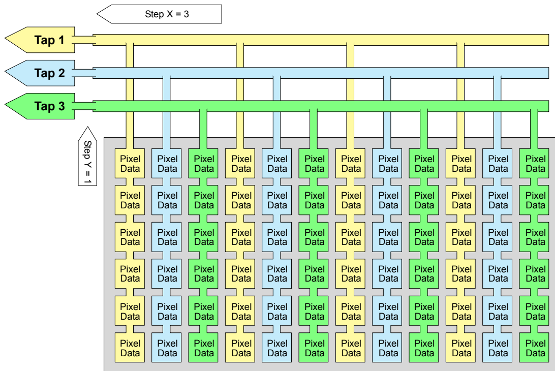
Fig. 41: 1X3-1Y Tap Geometry
