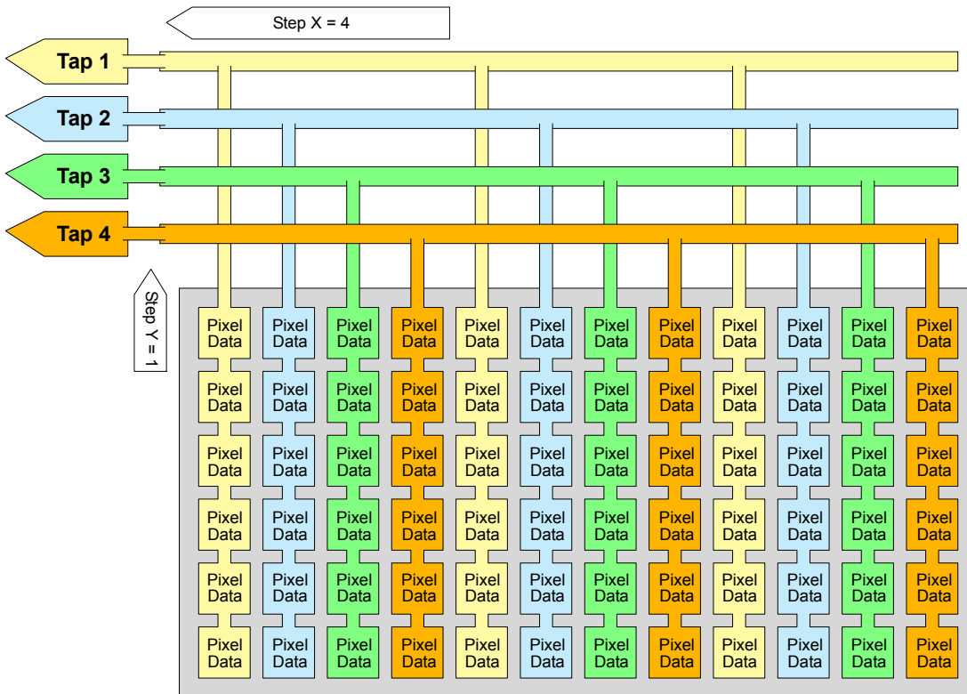
Fig. 42: 1X4-1Y Tap Geometry
